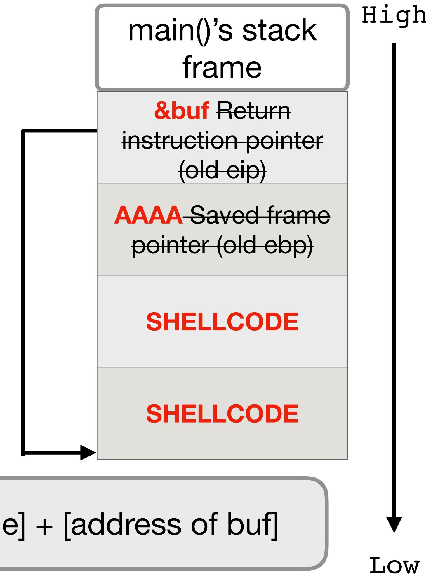
[8 bytes of SHELLCODE] + [4 bytes of garbage] + [address of buf]
